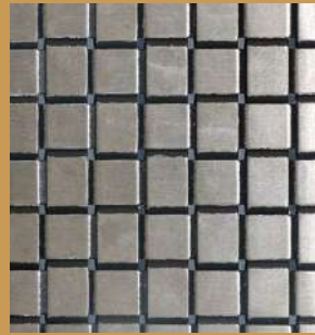
QKCWM-17 Warp Diameter:1.6mm Weft Diameter:1.7x4mm Warp Pitch:4.5mm Weft Pitch:4mm Weight:15.2kg/m 2 Opening Area:0%
