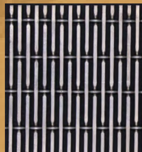
QKCWM-10 Warp Diameter:1.5mm Weft Diameter:2mm Warp Pitch:4mm Weft Pitch:17.5mm Weight:2.5kg/m 2 Opening Area:45.7%
